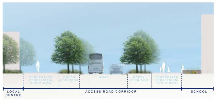
Figure 17; Typical section diagram of access road through the local centre
